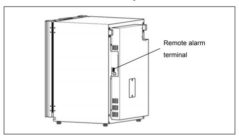
The alarm is outputted from this terminal. Contact capacity is DC 30 V, 2 A. Contact output:
